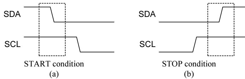
Figure 2 The START (a) and STOP (b) conditions are both initiated by the master. The START condition happens when the SDA line changes from a high to a low while the SCL line is at a high. The STOP condition happens when the SDA line changes from a low to a high while the SCL line is at a high. These are the only two situations where the SDA line can change when SCL is at a high.
